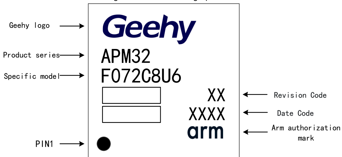
Figure 27 QFN48 Coding Specification
